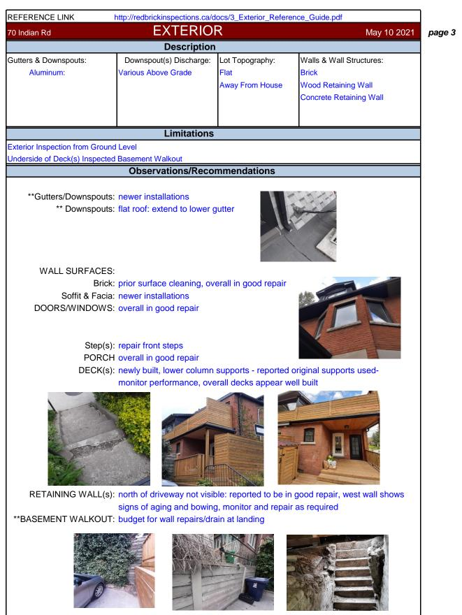
Note: Maintain Gutters & Downspouts annually. Extend Downspouts at least 6-feet away from the house \*\* Any or all these items may contribute to **Basement Leakage**. Please see Interior Form
